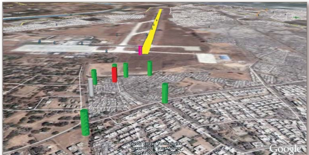
PIXEL SOFTEK's FME workspace requires only a few FME transformers to create a runway feature, as well as 3D obstacle features in KML, from a source dataset in AIXM.
